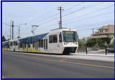
Light rail transit with exclusive right-of-way, Portland, Oregon
