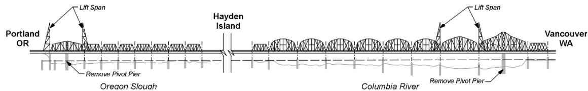
Both the Columbia River and Oregon Slough swing spans would have to be replaced with lift spans in order to allow the new alignment to run parallel.
